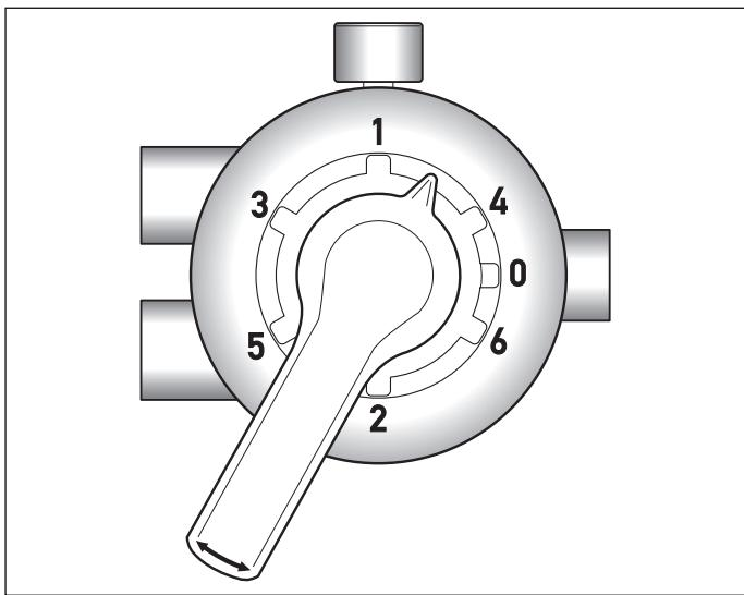
► **Backwash (2):** the water is driven by the pump and is carried in the opposite direction as in filtering, in order to clean the filter. In this case, the water enters the filter through the central tube, exits from the lower filtering elements of the internal distribution system, goes up through the filtering material and then exits from the attachment to which the drain pipe is connected, carrying with it the deposit trapped by the filtering mass during filtering.
