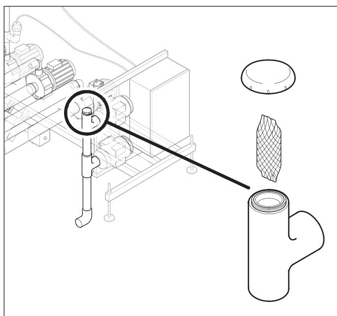
► If the blower is to be used for the aroma therapy treatment, insert the perfume cartridge in the blower connection pipe as shown. Once this cartridge is finished, it can be replaced by simply unscrewing the plug and replacing it with a new one (cartridges are available from authorised dealers and technical service centres).
