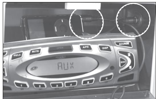
Connect the MP3 player to the external port with the RCA mini-cable provided.
